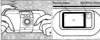
\*If the distance between the subject and the camera is set at 0.35 m (1.1 ft.), the picture area will be inside the close-up correction marks as shown in the illustration. Shooting range: From 0.35 m (1.1 ft.) to—∞(infinity)
